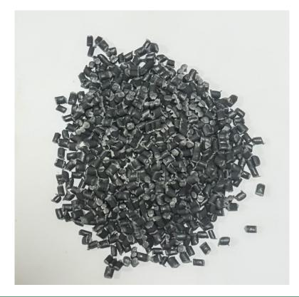
**TECHNICAL DATA SHEET** Recycled Low Density Polyethylene (LDPE) rLDPE [CASRN 9002-88-4]
